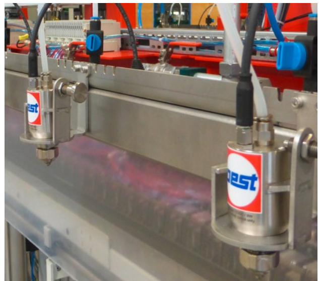
Water spray unit
