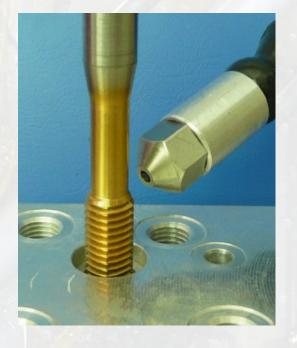
Oest Meba SP spray mist lubricants are formulated without mineral oils from components which offer maximum lubricating action with regard to the minimal quantities used. Oest Meba SP spray mist lubricants are compatible with non-ferrous metals and light alloys.
